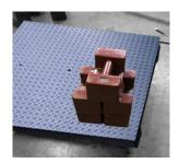
After calibrating, place a test weight weighing around 1/3 of the maximum capacity of the scale in each corner and take note each reading including the reading at the center of the scale (e.g if 1Klb max capacity, use around 325 lbs test weight).
