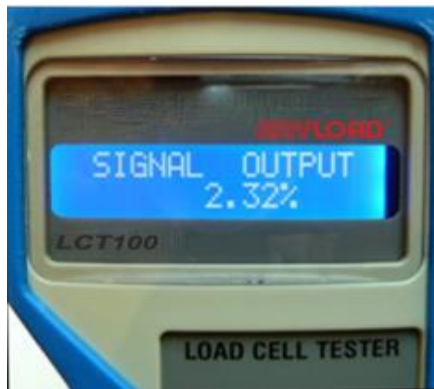
Figure 2 Zero output when load cell is loaded
