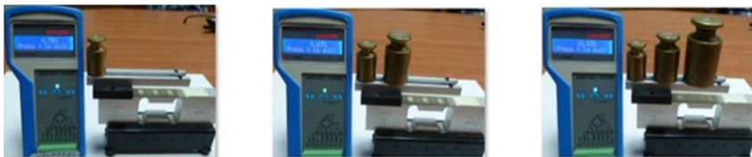
Figure 6 performing a linearity test with 3 weights
