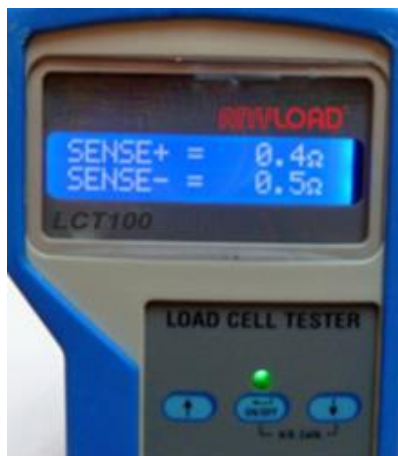
Figure 7 Typical reading when sense lines are OK
