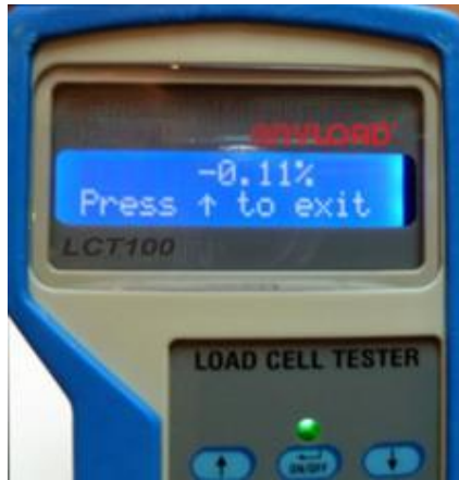
Figure 5 Typical reading when load cell is not loaded
