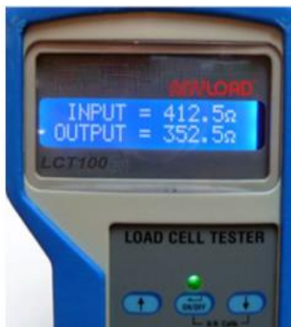
Figure 3 Typical bridge input/output results
