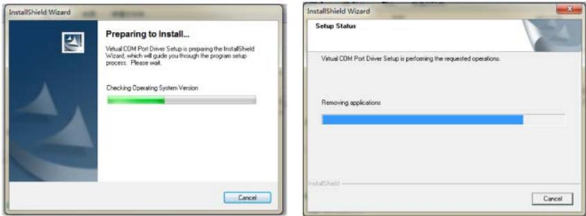
Once driver software is successfully installed, insert the USB cable with the P180 to the PC. The PC shall execute auto installation. You can open the device manager to check the virtual COM port for this USB. At the device manager (see the image below), telling that the driver was successfully installed.
