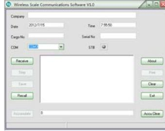
Set the COM port number based on the COM number assigned at device manager.
