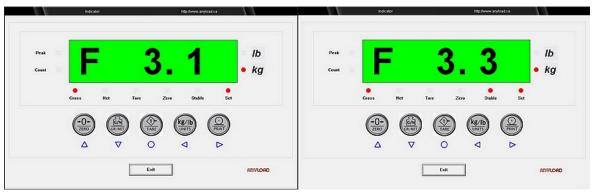
Go to F3.1 and F3.3 and follow the instructions in the manual to set the zero point and load calibration
