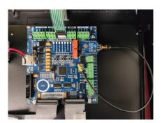
Install the antenna outside the unit at the bottom.
