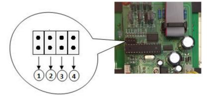
To change the channel for your BD Wireless Display you need at least 4 pieces jumper switch or 4 pieces push button switch with jumper switch at the end (see photos below)
