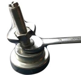
Lock the bolts of the AMF feet using two wrenches. One is at the jam nut and the other is to the fixed nut. During this stage, make sure the bubble level still remains at the center otherwise you need to adjust the feet again. After locking the bolt of each foot, you may check the reading in each corner against the reading of at the center if it has a big tolerance. If necessary to adjust, you may tune up the J04EA junction box again until the readings are almost identical
