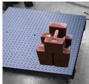
After calibrating, place a test weight weighing around 1/3 of the maximum capacity of the scale in each corner and take note each reading including the reading at the center of the scale (e.g if 1Klb max capacity, use around 325 lbs test weight ).
