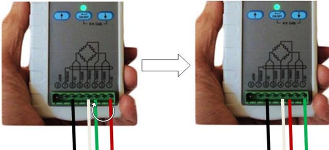
Run the tester using the full testing cycle. The input and output resistance results will be the resistances of the other pair of strain gages.
