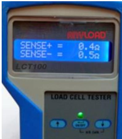
Figure 7 Typical reading when sense lines are OK
