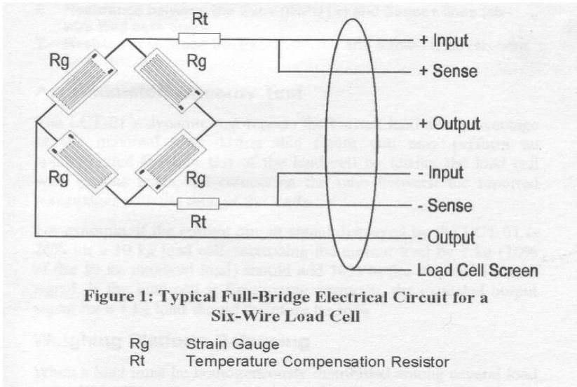
Figure 1 A typical scheme of 6 wires load cell
