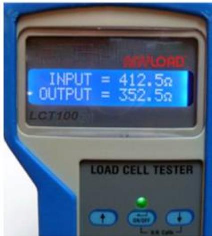
Figure 3 Typical bridge input/output results
