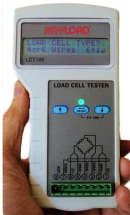
1. Connect the load cell cable to the right pins in the connector
