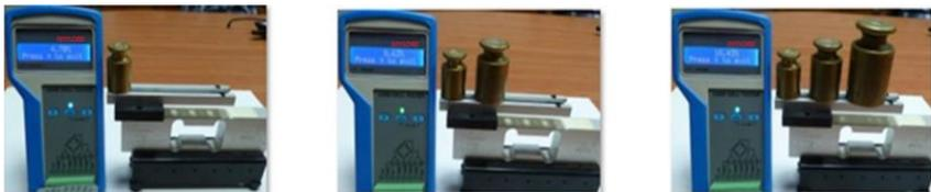
Figure 6 performing a linearity test with 3 weights
