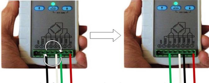
Run the tester using the full testing cycle. The input and output resistance results will be the resistances of a pair of strain gages.
