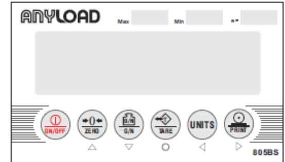
Press the [ON/OFF] button for 2 seconds. The indicator will start with self checking displaying digits 000000 to 999999. In the weighing mode, press the Zero button to return the scale to zero.
