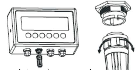
Connect the power supply. Insert the power supply male connector to the female terminal in the indicator. Push and turn it clockwise to tighten and lock. Refer to the image above.
